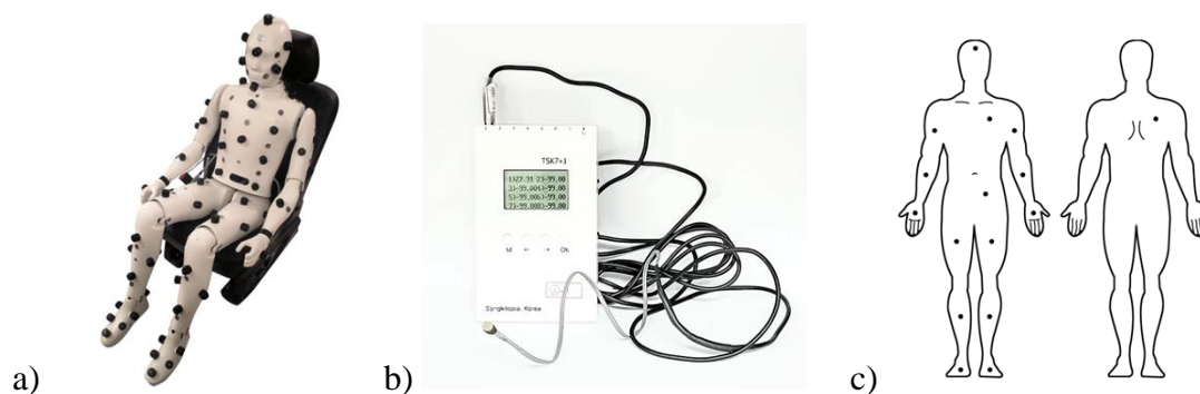
Figure 1. Instruments for the measurement. a) HVAC manikin for environmental parameters measurement, b) Sensors for T_{skin} measurement, c) Body parts where the T_{skin} sensors were attached
